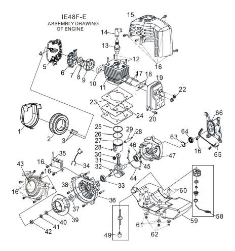
\*(Not Shown) AF-200 Cylinder Assembly (Parts 11, 12 and 23-46)
